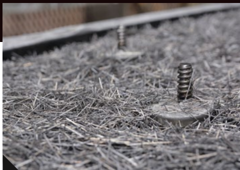
1 Fibres placed in position
