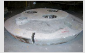
Monolithic roof of ladle furnace Voûtain de four poche
