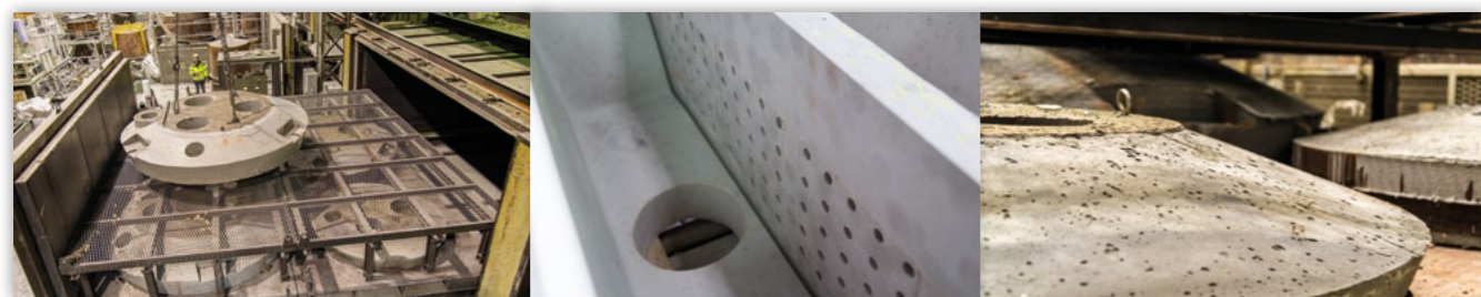
Precast pieces dried up to 450 °C. Small or medium serial productions, 10 kg to 20 tonnes weight unit. Precast pieces designed from specifications and from drawing of the customers. Refractory pieces manufactured from our high performance castable mixes selected to withstand according to demand thermal shock, high temperatures, chemical attack and/or abrasion. Our FibroCeram ® quality is requested in case of application with mechanical shocks and high temperature.
