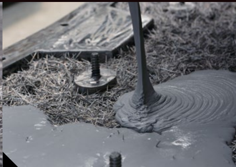
2 Matrix poured over fibres
