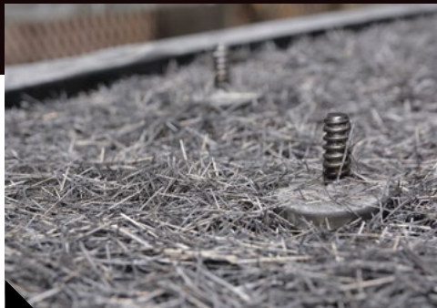
1 Fibres placed in position
